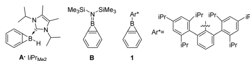
Scheme 1 Carbene coordinated benzoborirene A , bis(trimethylsilyl)-amino substituted benzoborirene B , and kinetically stabilized benzoborirene 1 .
