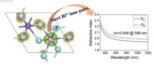
From BiF<sub>3</sub> to BiF<sub>3</sub>·H<sub>2</sub>O: diverse Bi(III) coordination for structural transformation and birefringence regulation
