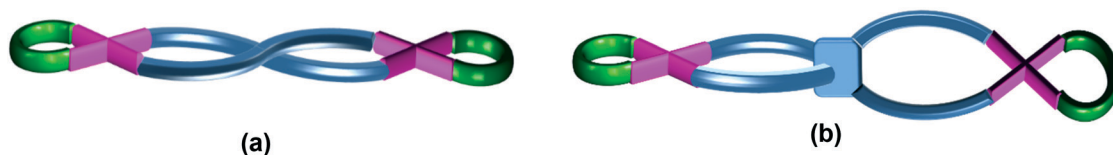
Fig. 7 Schematic representation of (a) a "helicite" complex formed from two bidentate ligands and (b) a "twisted" complex formed from one unit of a tetradentate ligand.
