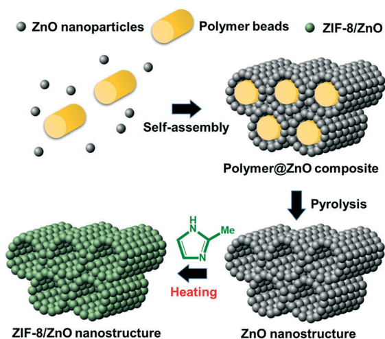
Fig. 1 Schematic description of the preparation of hierarchical ZIF-8/ZnO nanostructures.
